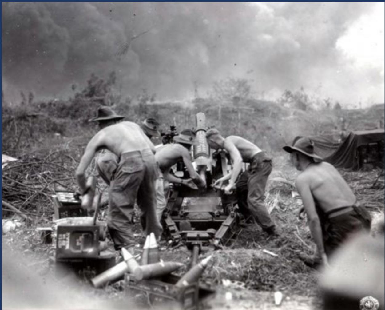
Above: Gunners of the 36th Siege Artillery Group, with a 9.2 inch howitzer, the heaviest gun operated by the RAA, with a range of 9,000 meters for it's 130kg shell.
