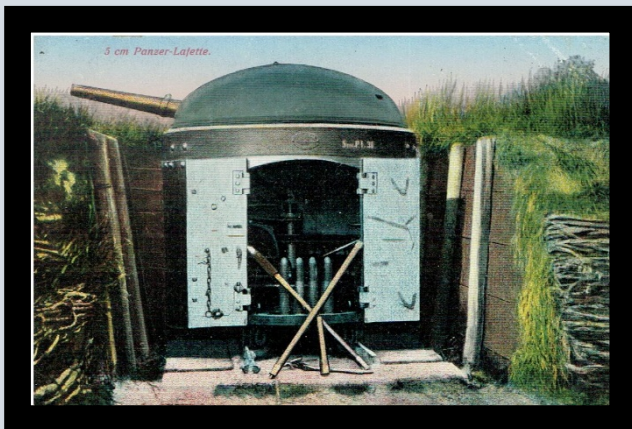
Figure 3. An August 1917 postally dated postcard of a German 5-cm gun in mobile armour carriage employed as an anti-tank gun on the Western Front. Actually of 5.3-cm in calibre, the Model 1887 L/24 gun was mounted from about 1890 in German fortifications. In these it was normally housed in a shellproof concrete shelter and moved into its emplacement along a set of rails when it was required to come into action. (Author's collection)
