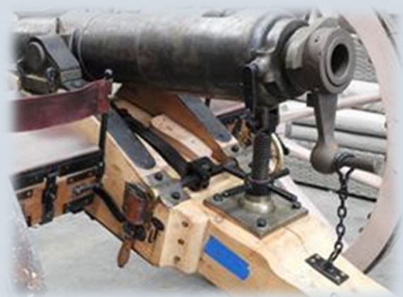
View of the breech, elevation and traversing mechanism with azimuth nut.
