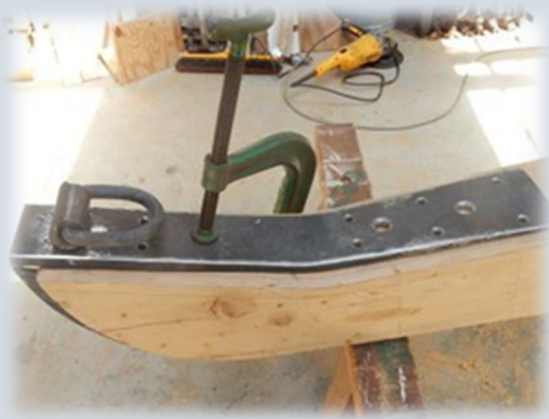
Trail plates being fitted, Nov. 2017.
